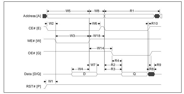
Figure 25: Write-to-Asynchronous Read Timing
