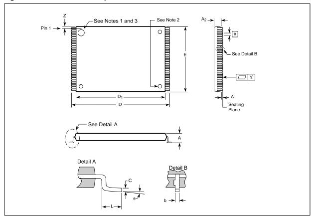
Table 3: TSOP Package Dimensions (Sheet 1 of 2)
