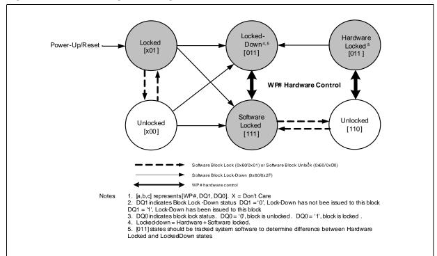
Figure 6: Block Locking State Diagram
