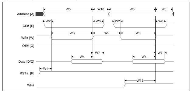
Figure 23: Single-Word Write Timing
