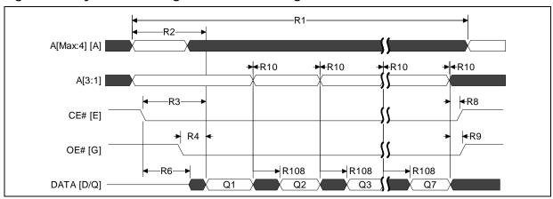
Figure 22: Asynchronous Page Mode Read Timing
