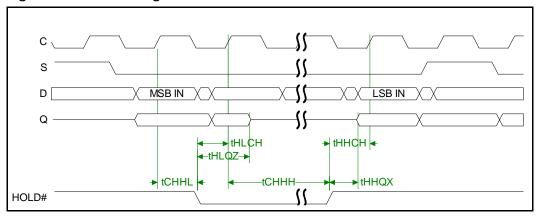
Figure 29: Output Timing
